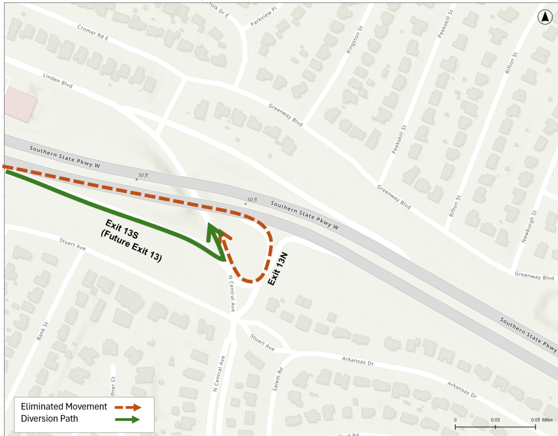
Figure 6.1.1 – Diversion Path for the Eliminated Exit 13N Ramp
